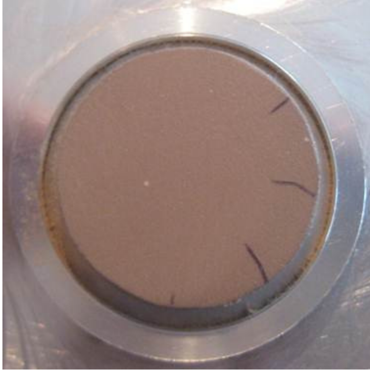
As the foot gets flatter, the sanded area is growing. 50 more circles...
