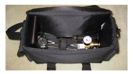
Fill the space in the soft case over the regulator with bubble wrap or 'air bags' to keep the meter seated at the bottom of the case.
