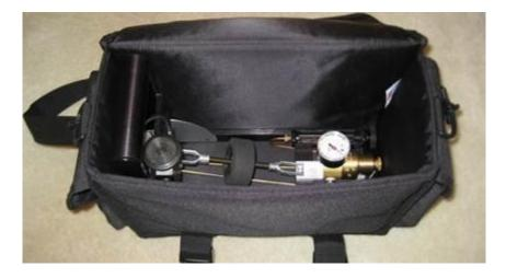
Fill the space in the soft case over the instrument with bubble wrap or air pillows to keep the meter seated at the bottom of the case.
