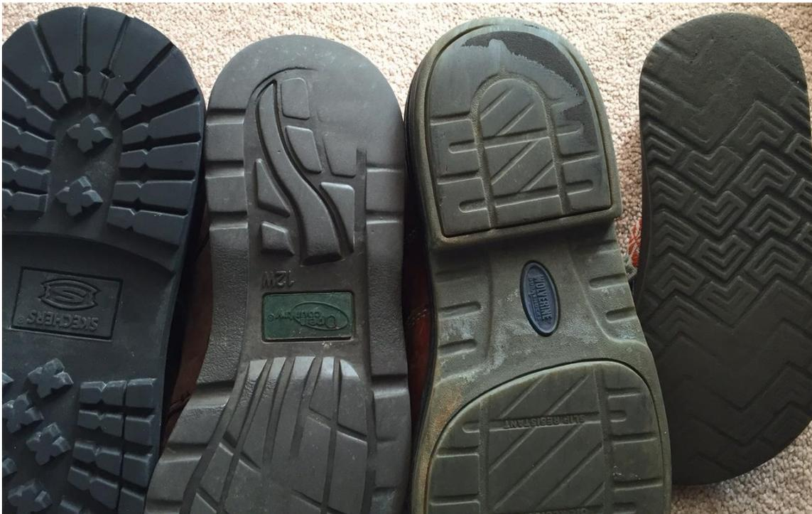
When using a tribometer to evaluate the relative safety of walkway surfaces, the test foot needs to be representative of the foreseeable footwear in a slip injury event. As can be seen from the photo, it is highly likely that the **heel contact area** of foreseeable footwear will have **little or no tread**. This is particularly evident with footwear involved in slip and fall injury events, even when there may be prominent tread on the balance of the bottom of worn footwear.
