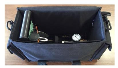
Fill the space in the soft case over the instrument with bubble wrap or air pillows to keep the meter seated at the bottom of the case. Your calibration tile and sander should be bubble wrapped and placed in the same packing box, but not in the soft case compartment with the meter.
