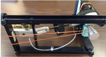
Put the slipmeter in the soft case with the mast set to 0.05 slip resistance on the protractor (nearly vertical).
